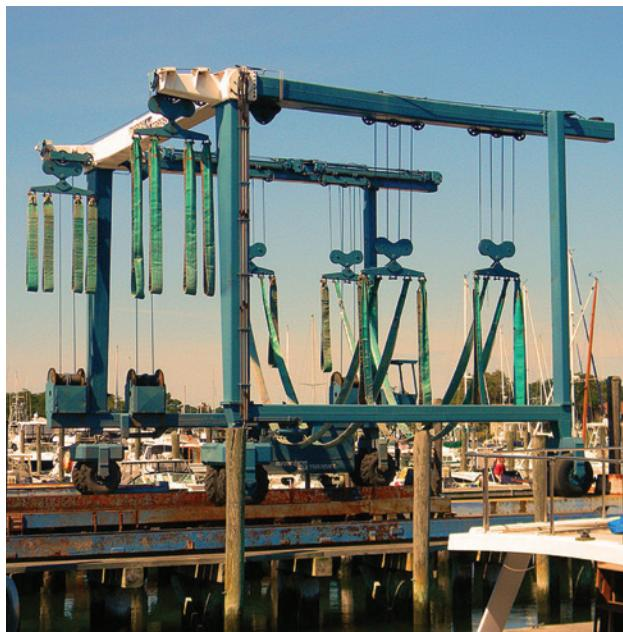
Boat Lifting or Marine Lifting Slings are designed to help you conveniently lift any boat. Choose from Single or Double Ply slings with Widths up to 12". Lift up to 53 tons when pairing slings and rigging in a Basket Hitch.
