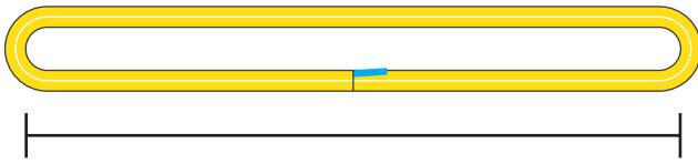
**Matched Set Length Tolerance:** When multiple legs of a bridle sling are made, or when multiple slings are prescribed to be made within a Matched Set Tolerance, their length variance from their nominal length shall remain within a dimension equal to one-half of their corresponding Standard Length Tolerance Values.
