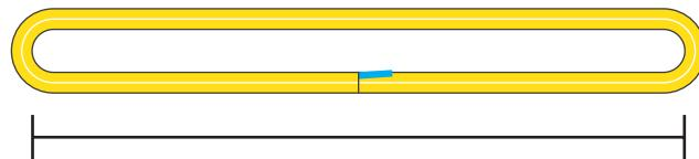
**Measurement Method:** Roundsling length is measured with the sling laid flat while being manually pulled taut.
