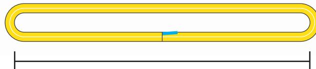
**Matched Set Length Tolerance:** When multiple legs of a bridle sling are made, or when multiple slings are prescribed to be made within a Matched Set Tolerance, their length variance from their nominal length shall remain within a dimension equal to one-half of their corresponding Standard Length Tolerance Values.
