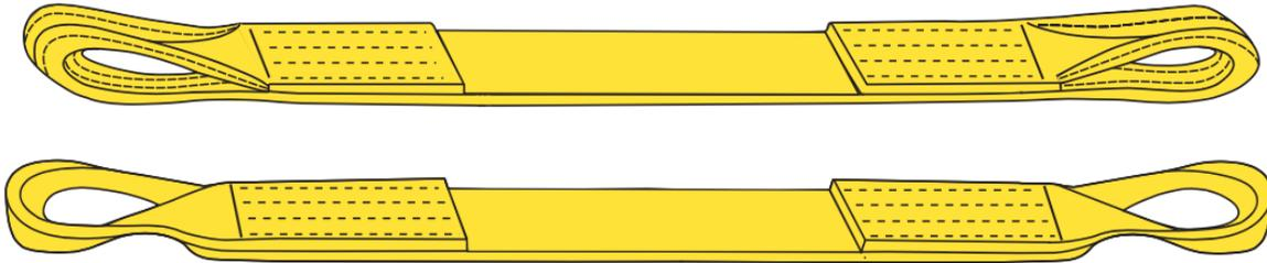
Eye and Eye slings can be used in choker, vertical and basket hitches. Slings with Half Twist (Type 4) eyes are furnished unless Flat (Type 3) eyes are specified. Sling eyes will be wrapped at the bearing point unless otherwise specified.
